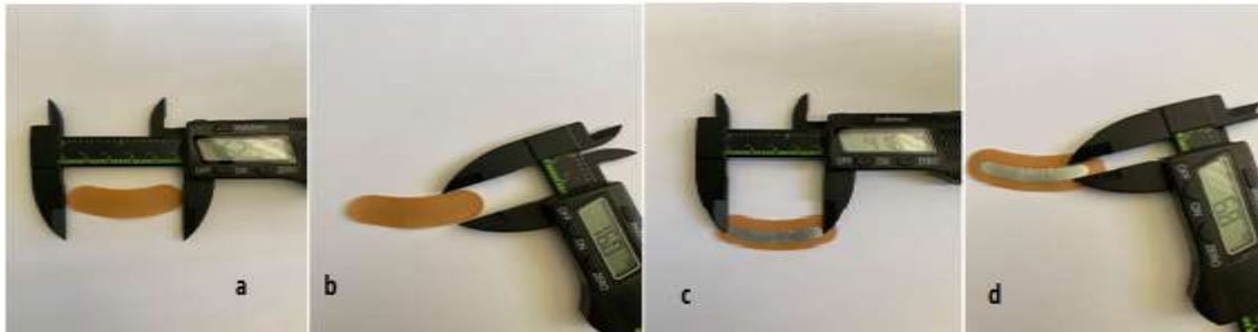
Figure 1: The wearable patch includes a flexible substrate, a binder an adhesive layer, with an electrode foil attached to it. Zinc foil thickness 0.025mm and Copper foil thickness 0.025mm.
