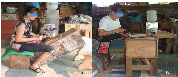
Figure 5: The original or conventional workstation with sloping work surface (A) and a tilting adjustable desk and stool prototype (B).
