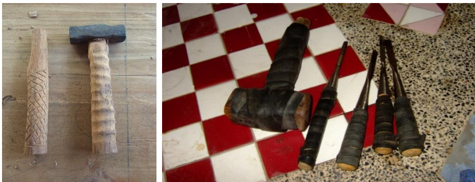
Figure 4: Hammer handle with grooves for fitting fingers (left) and rubber wrapped around hammer head and/ or handle and chisel handle (right).
